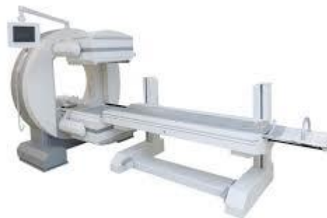
Gamma camera to study the function of kidney, liver, and lungs.
